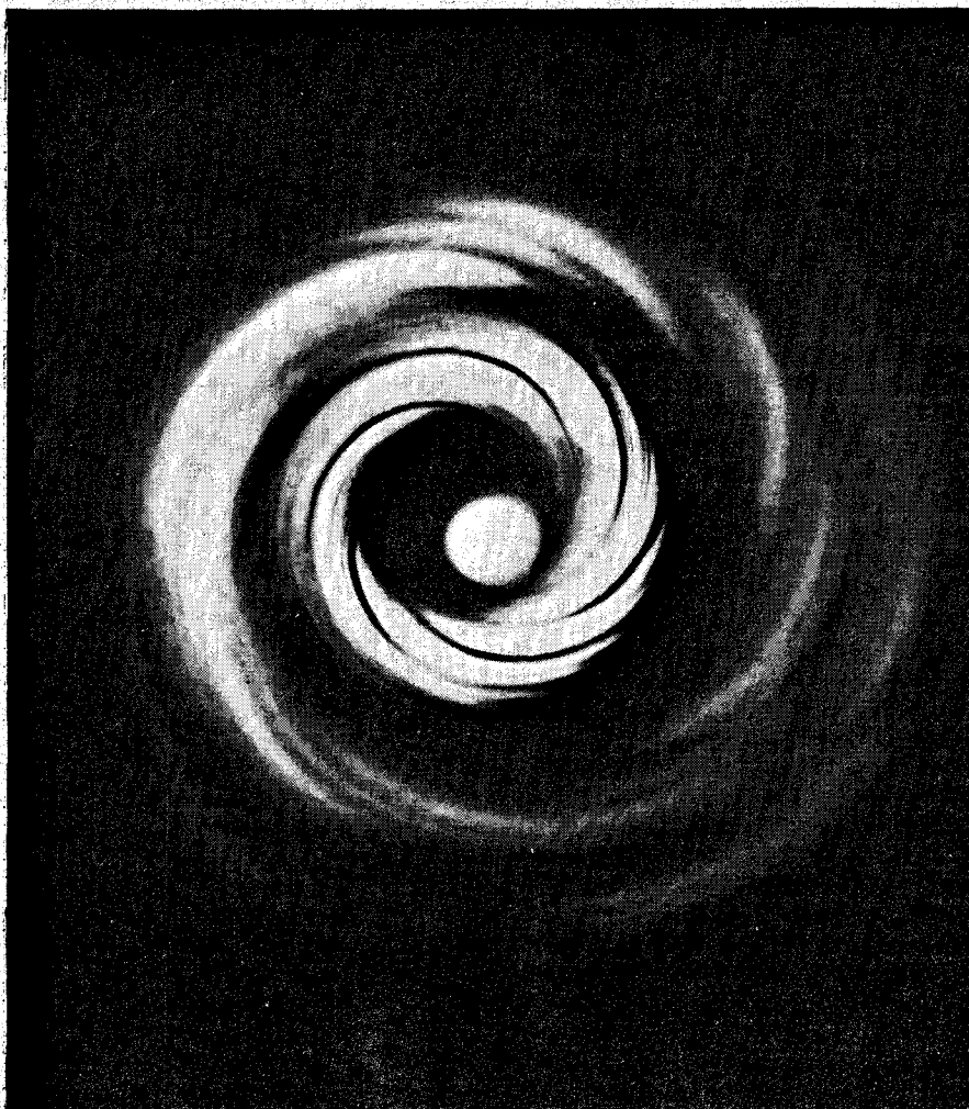
This is neither a scene from "2001" nor a satellite's view of the eye of a hurricane. It's a glimpse down a rifle barrel illuminated at the chamber end by a Corning Flexiflash fibre optic unit. The unit is proving useful for gun enthusiasts in examining rifling, the chamber, the wear in the barrel's throat — all areas that can effect a weapon's accuracy.
