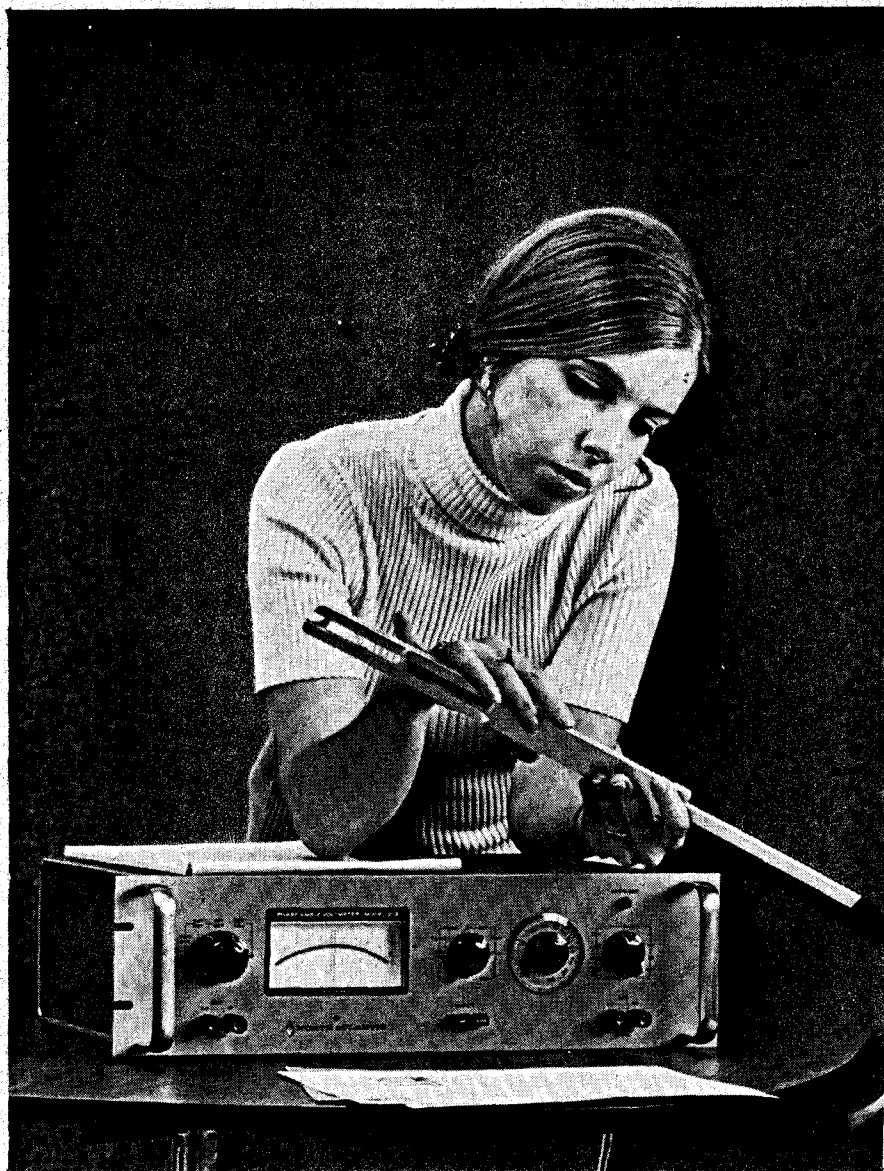
Our lead picture shows North Atlantic Industries Model 213 solid state phase angle voltmeter. The instrument measures in-phase voltage, quadrature voltage, and phase angle, relative to an arbitrary reference voltage; uses a built-in filter to measure the harmonic-free "fundamental" component of input voltages; and bypasses the filter to measure "total" input voltage (as with an ordinary ac voltmeter). The meter may also be used as a phase-sensitive null detector with a two micro-volt resolution. The manufacturers are represented in Australia by Ronald Payne Pty. Ltd.
