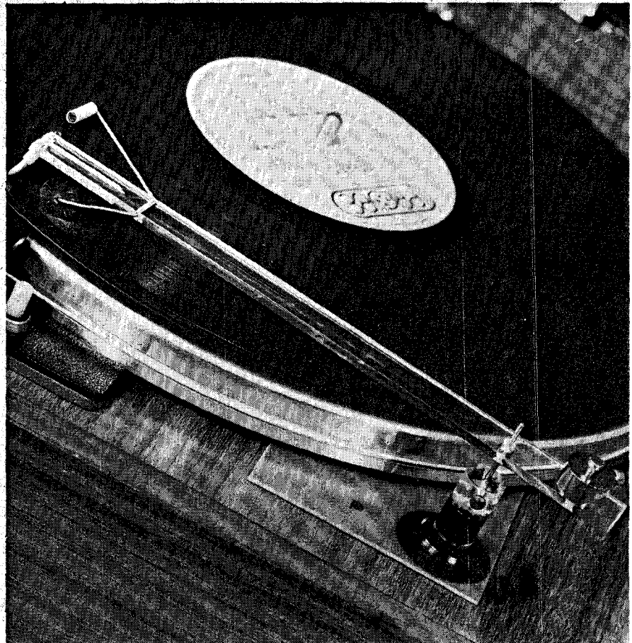
A 'Dust Bug' can be easily fitted to any turntable — this simple attachment continually cleans the record during playing.
