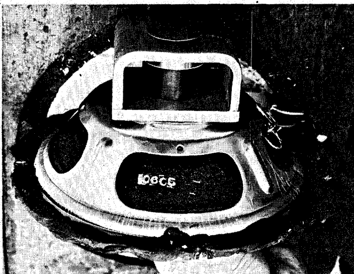
These two photographs dramatically illustrate the long voice coil of the AR-6 bass driver. (Note the open yoke construction of the magnet assembly).
