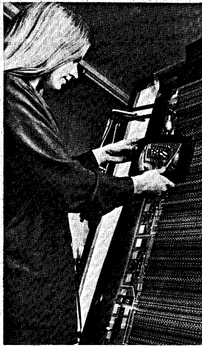
RIGHT: Physical inspection of rubyliths of a 1,024-bit shift CDI register. LEFT: An operator carrying out a process control check using a curve tracer which shows the collector-emitter characteristics of a CDI transistor in a digital array. BELOW: View of part of the pre-production line for CDI bipolar integrated circuits in the Electronics Department of Ferranti Ltd.
