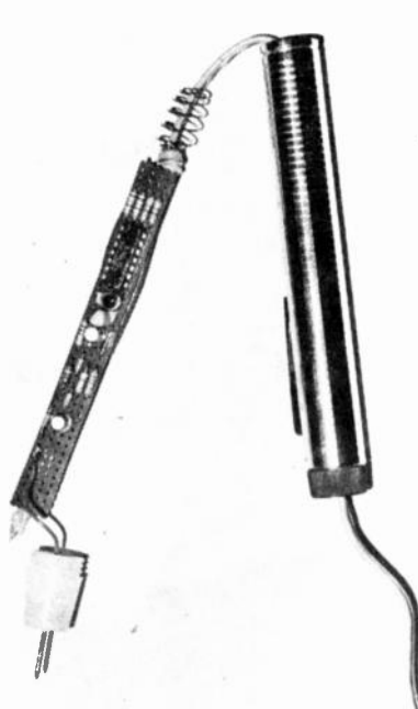
How prototype unit was constructed; the circuit board should be insulated from the metal case.
