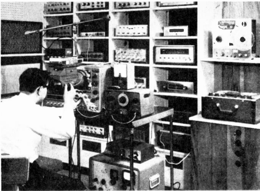
Test setup that was employed for qualitative display of speaker distortion.
