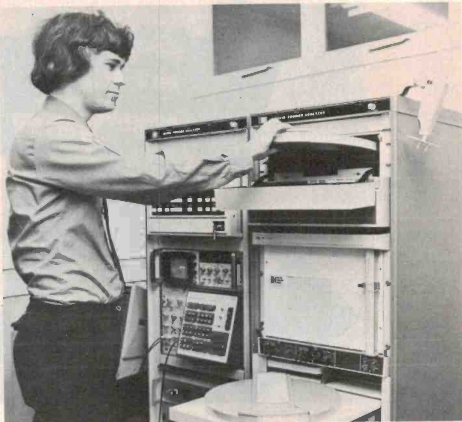
Computer analysis of speaker designs is being increasingly used by speaker manufacturers. Here, an engineer loads a Fourier analyzer machine at the British factories of KEF Electronics.
