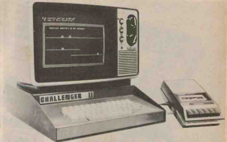
Ordinary, inexpensive cassette recorders are used to store programs 'permanently' on tape.
