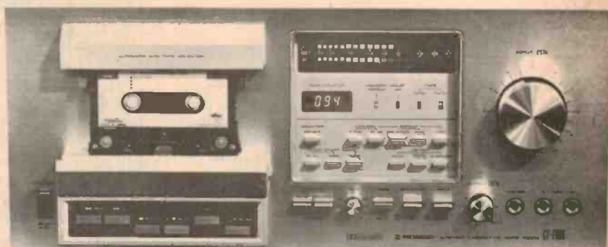
Pioneer's new CT-F900 micro-processor controlled cassette deck has all-electronic three-head transport system.
