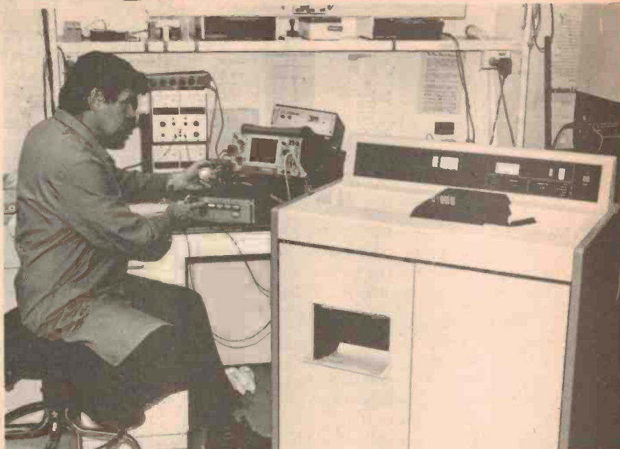
Mr. Graeme Mann, 3M Australia graphics system engineer, checks the response time of the simultaneous facsimile broadcast equipment.
