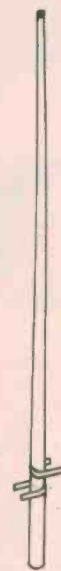
Figure 2. This base antenna, model CB470 made by Scalar, has a genuine gain of 6dB over a half-wave dipole and provides an increase in the effective radiated power of four times omnidirectionally. Overall height is 2.44 metres.
