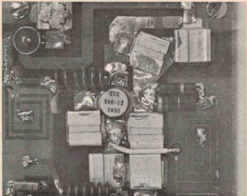
Close view of the output stage showing the placement of the metal-clad mica capacitors and RF chokes. Note the jumper from Q3 base to printed RF choke, RFC3.
