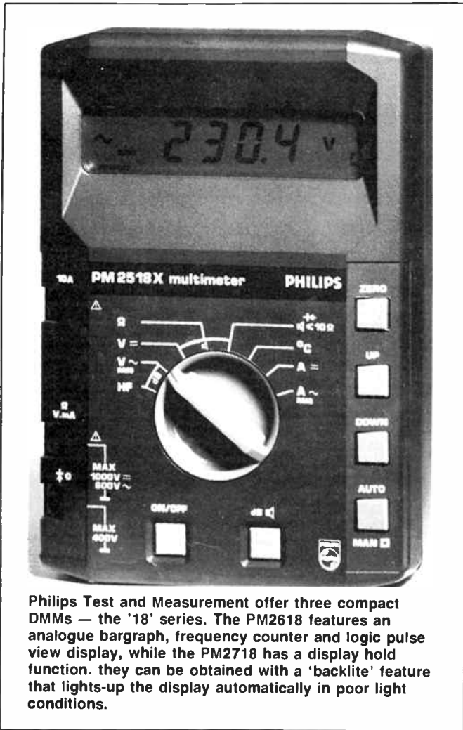
Figure 6. If you have a meter with a 'display hold' facility, voltage drop checks are much simplified. Clip the leads across the connection to be measured, select the function and set the meter to read millivolts (mV). Crank the engine and the meter will 'hold' the reading until you return.
