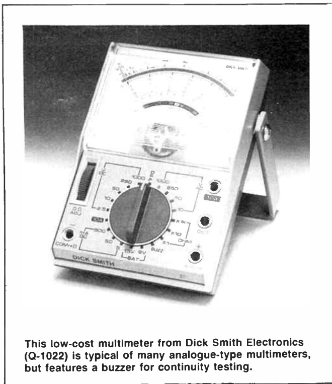
Figure 8. Check condensor leakage with your meter's resistance range. First momentarily short the condensor's two terminals to dissipate any residual charge, then attach the probes. Initially, it will show zero resistance, quickly rising to infinity. Any other indication shows you should replace the condensor.
