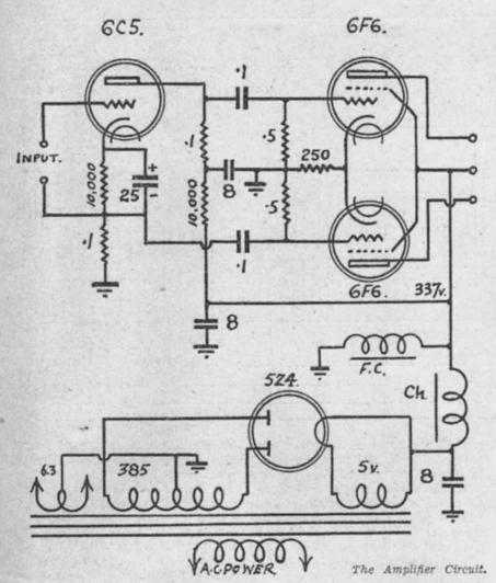
The power transformer has a secondary with a 150 milliamp rating, and should have a voltage rating of 350. Actually the original was built up with a transformer rated at 385 volts at 150 milliamps, but voltages worked out dead right in practice.
