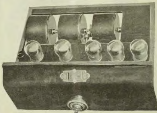
View of inside of drawer showing Rotoformers.
