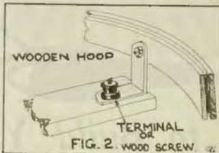
Attaching the hoop holding the cone paper to the unit standard.
