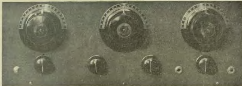
This is a view of the front of the panel. Note that vernier dials are used.
