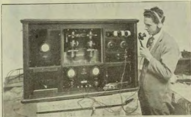
Testing the radio telephone apparatus to be used to connect Clifly Island Lighthouse to the mainland. The set has a transmitting power of 250 watts, and is simply operated.
