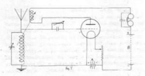
to the filament, thus giving rise to amplified impulses of current in the anode circuit in which are placed the telephone or loud speaker. We now come to the last of the three functions of the valve which was mentioned earlier, viz., rectification.
