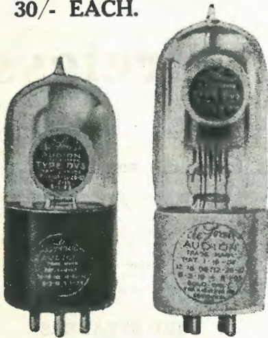
D.V. 3 Filament, 3 Volts, .06 Amp. Both Types Fit Standard American Socket. D.V. 2 Filament, 5 Volts, 25 Amp.
