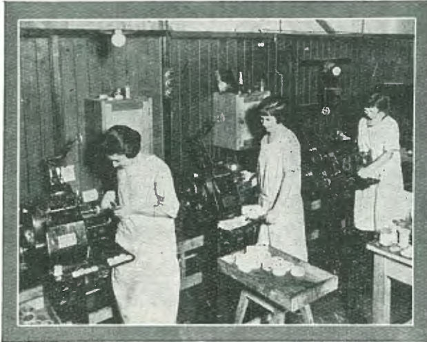
Making Honeycomb Coils by means of automatic winding machines.
