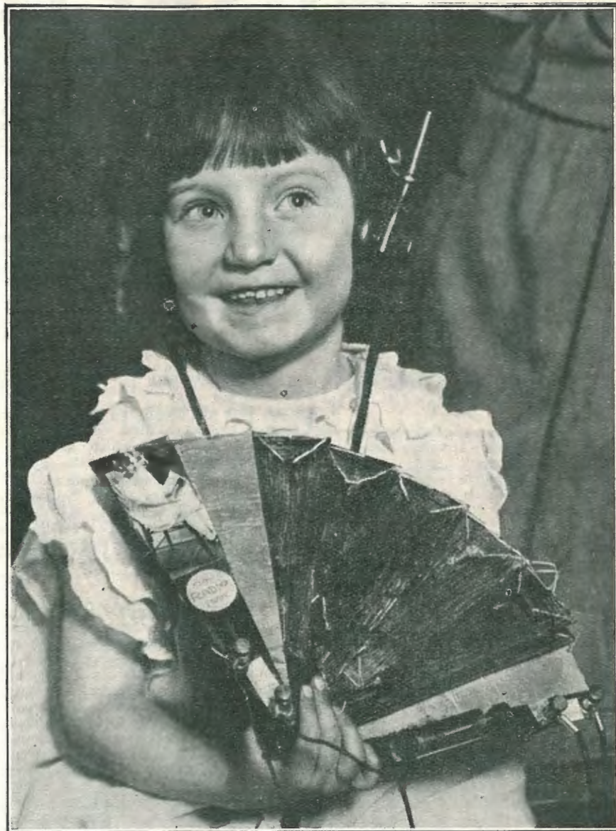
A real Radio "Fan." The coils of the Set are wound in the Leaves of the Fan and correct tuning is secured by either Opening or Closing it. A small Crystal is mounted on one of the end leaves and this little Set, although quite a Novelty, has proved itself as effective as a good many other Crystal Detectors.
