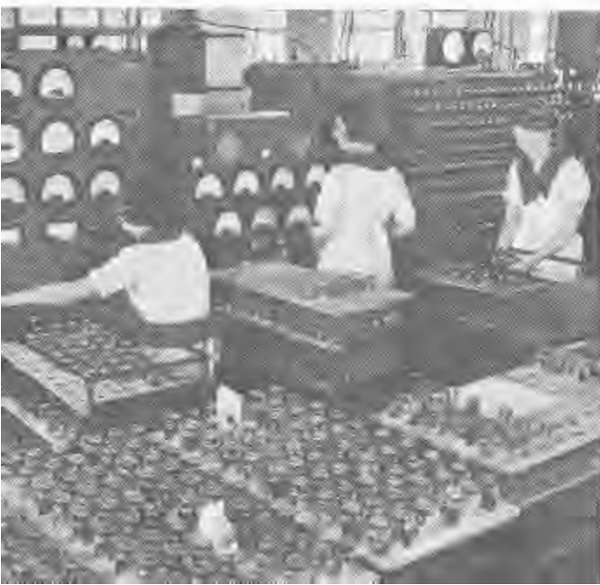
(K) The capping mill where the base is baked onto the glass bulb.
