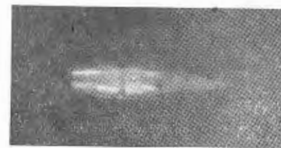
Fig. 10.—To take this light picture of a bullet in flight the X-ray tube was removed and the surge generator discharged across a gap to give an intense but extremely brief light.
