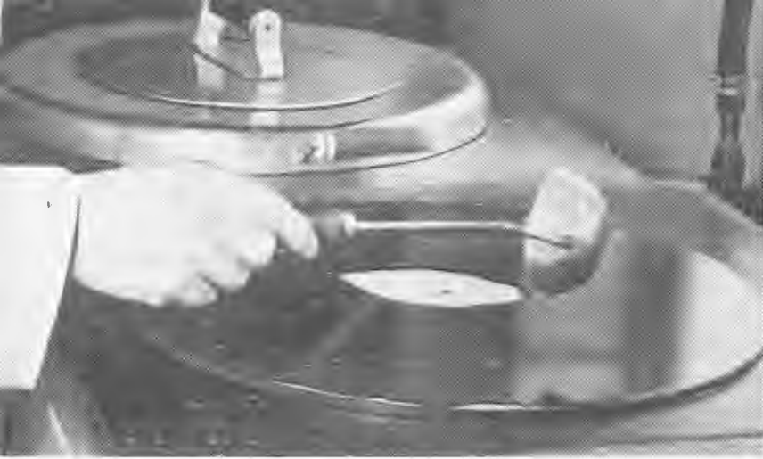
A.—Applying liquid wax to heated glass disc.
