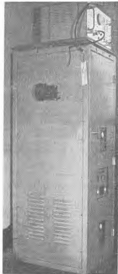
MTR master station equipment. The sub-modulator is at the top and the modulator and oscillator within the cubicle.
