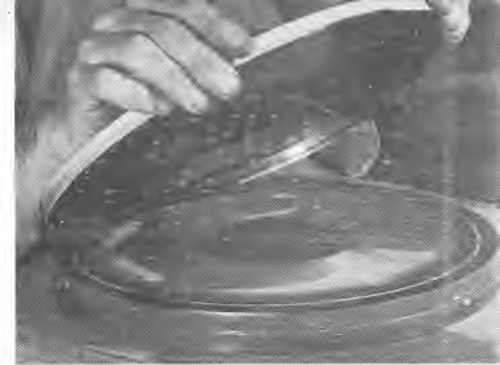
D.—The negative "shell" is carefully stripped from the wax.
