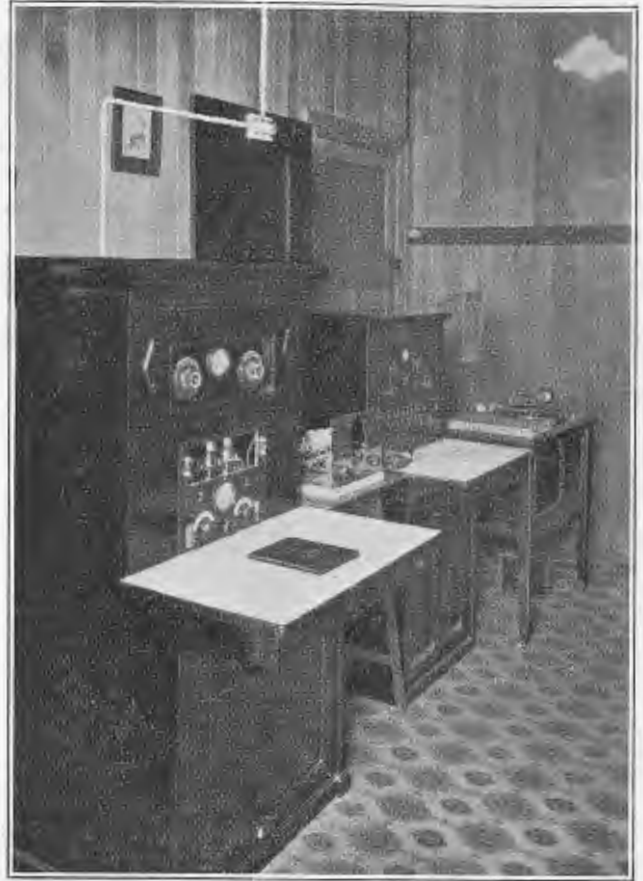
The Upper Photograph shows the Transmitting Apparatus at 4RM. From left to right may be seen the main 250-metre transmitter, the "baby" 32-metre transmitter, modulator and speech amplifier with the control panel, and the phonograph with its electric pick-up. The batteries are housed under the main transmitter.
