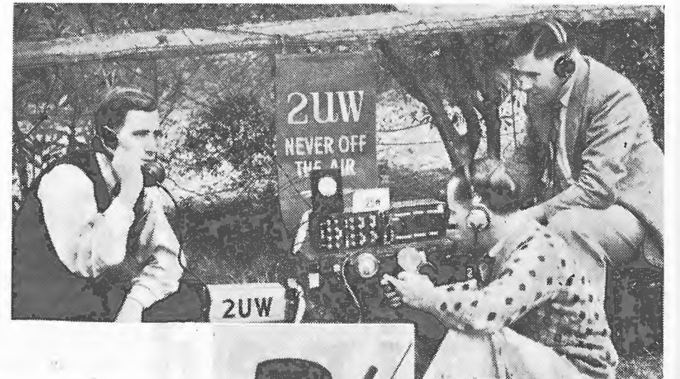
Since publication of the story ("Walkie-Talkie Golf Coverage," p. 28, "C.B.," Oct. 3) of 2UW's mobile broadcast cover of the championship golf at Rose Bay, Sydney, the accompanying photos of the equipment have come to hand. Above is shown the central transmitter-receiver, with special line-switching and patching gear to feed the 2UW line and the local sound system, in charge of technicians Austwick, Stephenson and Pearson, while inset at left is a close-up of Keith Dunbier, 2UW's sporting commentator, interviewing one of the competitors with the aid of a 5lb. crystal-controlled 5780 kc/s. transmitter-receiver. Ex-Army readers will have no difficulty in recognising the basic equipment employed.
