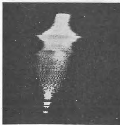
Illustrations of "Christmas Tree" reflections from the surface of frequency-run records. Top, aluminium disc produced by Fairchild-Proctor, showing flat response to about 6000 cycles. Middle, experimental acetate cut showing pronounced peak at 2000 cps. Bottom, same, made with adjustments to throw peak up to 6000.
