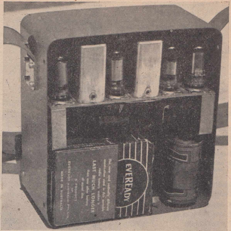
Replacement of batteries is easy when the back is removed, as shown here.
