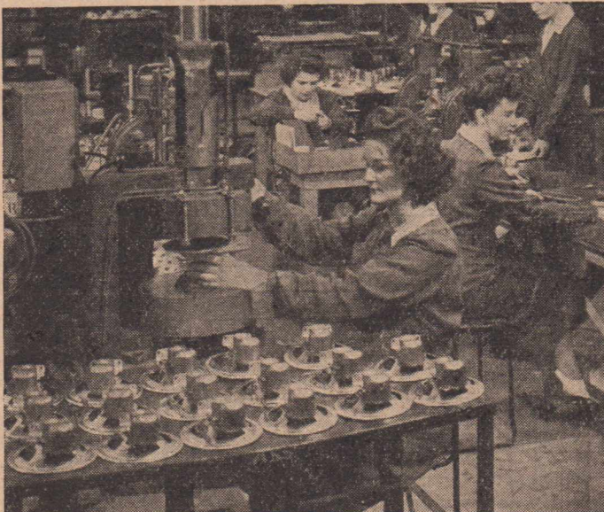
Rola speakers by the thousand . . . one of the last operations in the speakers' manufacture is the final magnetising process.
