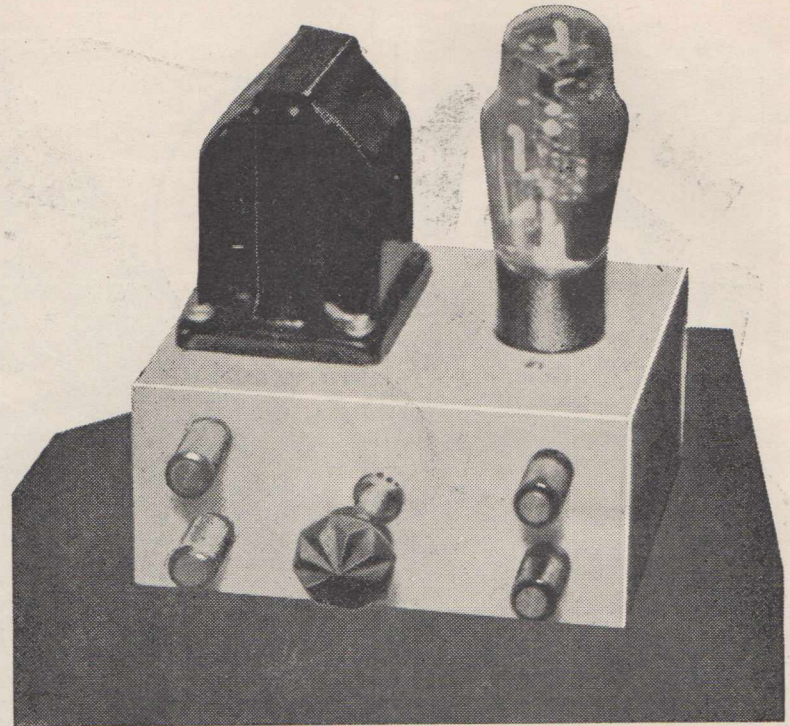
Only a handful of parts, most of which will be found in the junk box, are needed to build this code practice oscillator.
