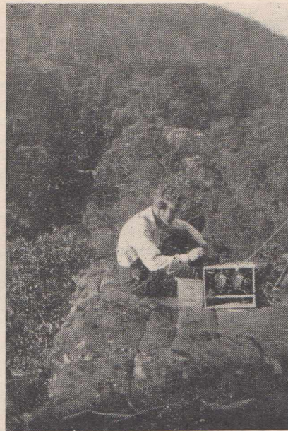
VK2LR-X, inland station, Operator VK2ACS. Transmitter is single stage S.E. rig, operating off 60 volts of "B" battery.
