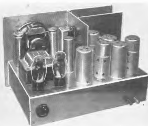
Front and rear views of the six-valve a.c. communications type superhet. reviewed below. Two i.f. stages are used.
