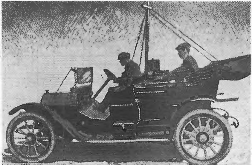
The latest in car radio—in 1916. During the war radio engineers spent much time developing mobile wireless equipment for use behind the lines, and this photograph shows an experimental radio-equipped car.
