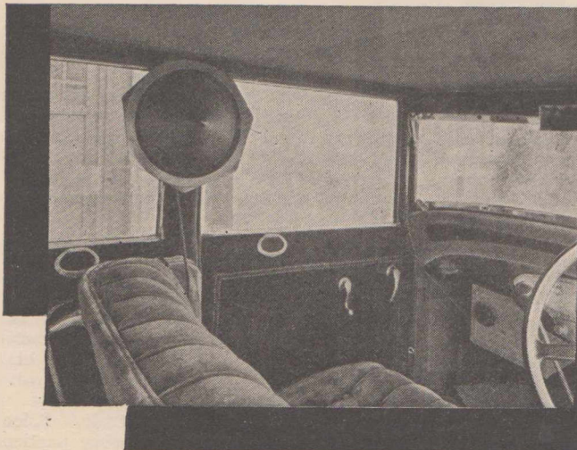
"A drawing room on wheels." In this case the controls are on the set itself and the speaker, a "Baby Grand," hangs from the door-post. The speaker may be alternatively mounted inside the roof.
