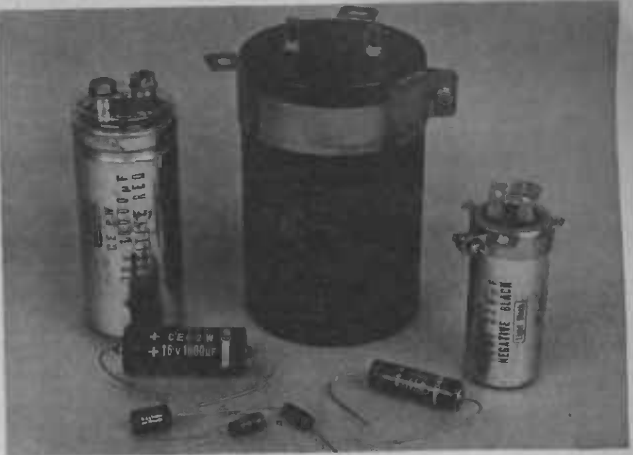
A group of modern electrolytic capacitors. The largest unit has a capacitance of 8000uF and a voltage rating of 75. The smallest units at the front have much lower capacitance ratings — typically 100uF or less, as well as lower voltage ratings.
