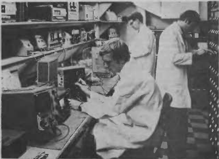
This service department, operated by a distributor of high fidelity sound equipment provides an object lesson in tidiness and organisation. Test equipment is ranged on shelves above the workbench, while the lighting is bright but even. Note the drawers at right for holding spare parts and drawers under the bench for cables and manuals. Not only does an orderly situation save time in the long run, but it encourages a better standard of workmanship.
