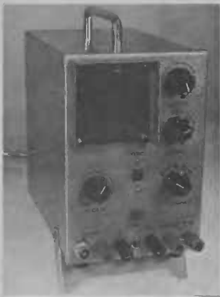
Fig 2: (above) Basic operation of the CRO or "scope". The horizontal plates are shown connected to the time base or sweep circuit and the vertical plates are connected to the circuit under test. Shown at left is a typical small instrument of this type. Note that the vertical amplifier control is calibrated in volts per centimetre sensitivity and the time base in milliseconds and microseconds.
