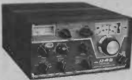
A Drake model R-4B receiver, especially designed for use by amateur radio operators. It employs valves, transistors and IC's.
