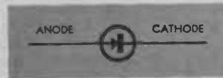
Fig. 9 (above): The usual schematic circuit symbol for a semiconductor diode.
