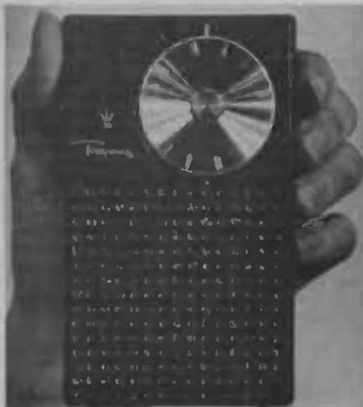
Exterior and interior views of a "personal portable" transistor receiver. Receivers of this type use the superheterodyne principle, and have from six to eight transistors.
