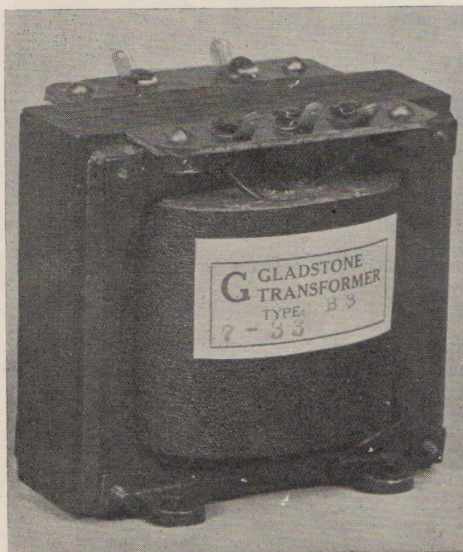
This is the input transformer — actual size.
