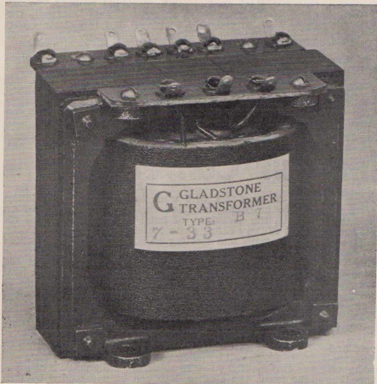
This speaker transformer is reproduced actual size.
