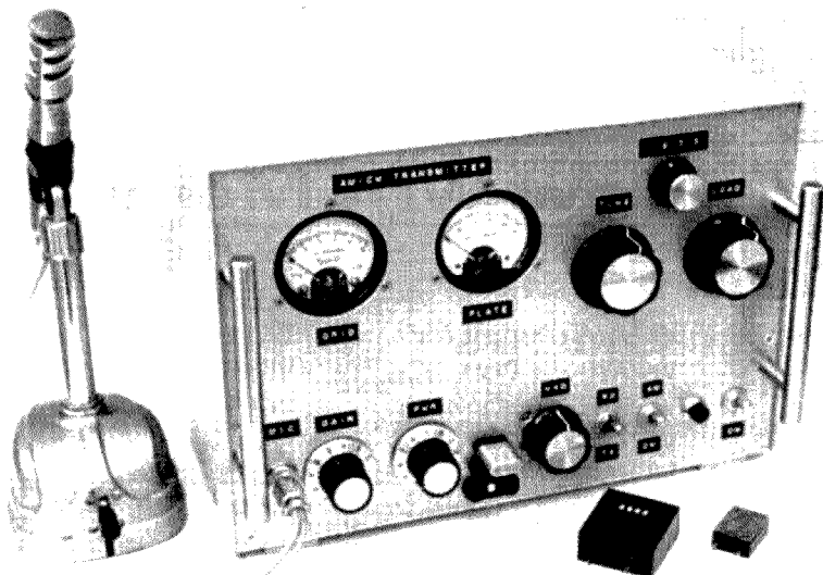
Photo 1. 25W AM/CW Transmitter
