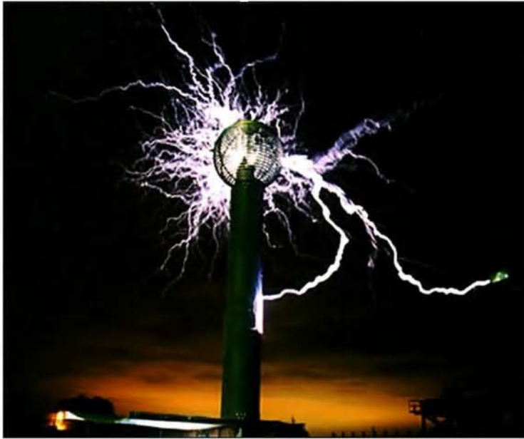
15 metre Electrum tower strike at near full power; E Orr is sitting inside electrode. (Photo by J Decker)
