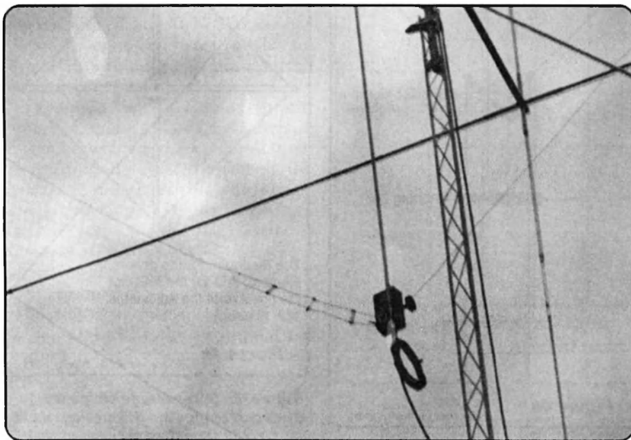
The driven element showing the gamma wire, feedpoint and coaxial choke
