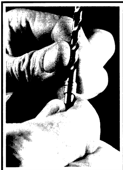
Wind the coils on a 5 mm drill.
