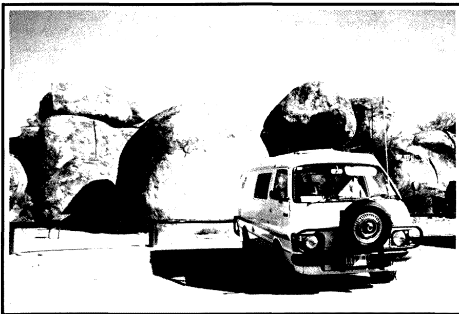
Ron's Hiace van parked at The Devil's Marbles in the Northern Territory. The Hustler antenna is mounted on the bull bars to the passenger's side of the spare wheel, and the Global whip is gutter mounted over the passenger side front door.
