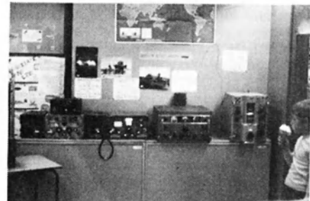
Left to right — C45 with power supply and B47 on top, C11 transmitter with power supply, AR88 and B40.
