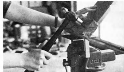
Dress the metal with a hammer to form a right angle.
