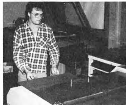
Feeding the Exposed Plate into the Automatic Plate Processor.
