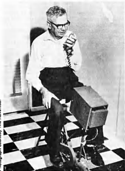
Alf Traeger and a later model Pedal Wireless. The photograph was taken in February 1963. Twenty of these sets were sent to the African Flying Doctor Service by Traeger.
