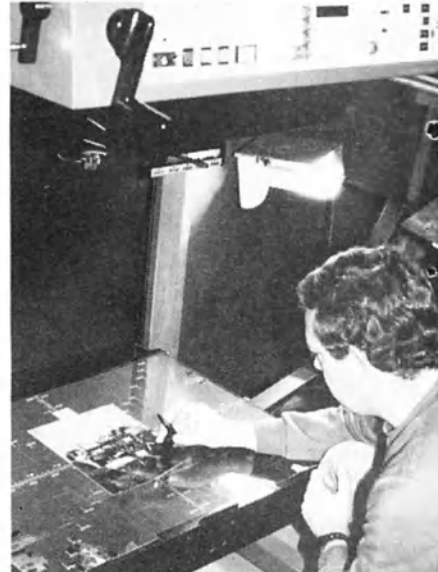
Setting up the Process Camera to make a Screened Bromide.
