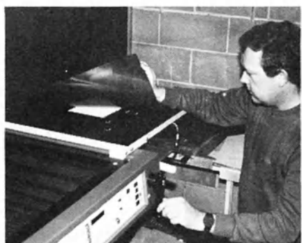
The Camera Operator applies the grey screen to the Bromide Negative.
