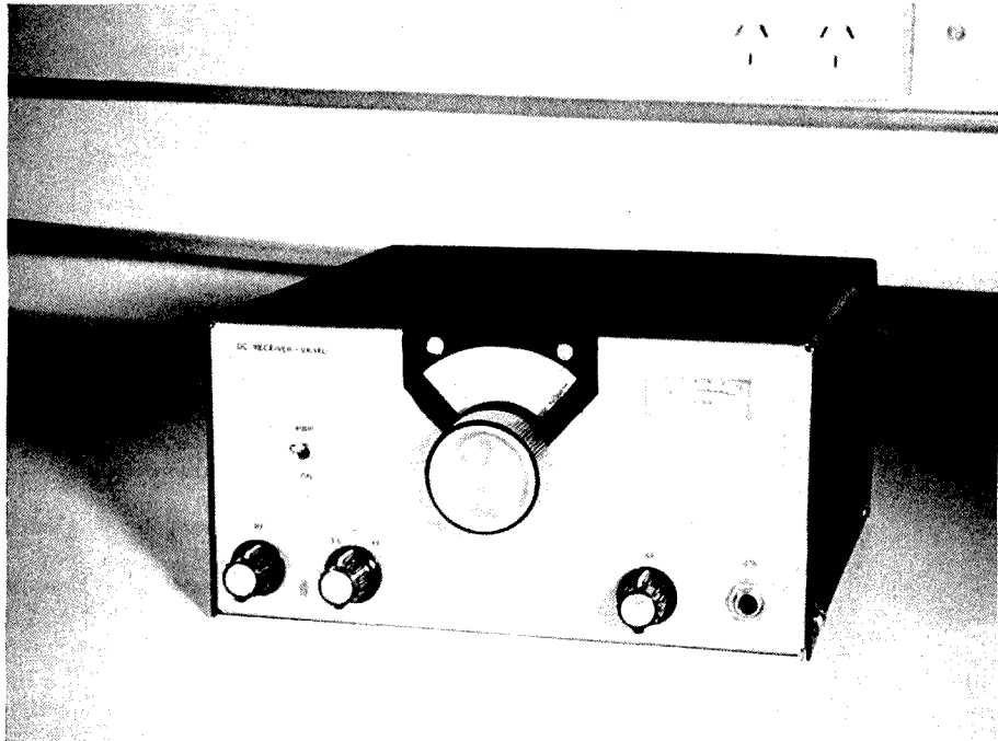
Completed DC Receiver.
