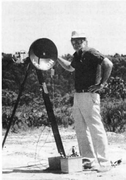
Dick operating his 10 GHz narrow band FM transceiver.
