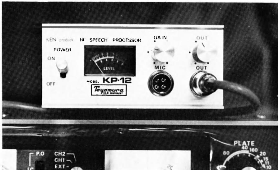
Ken products are produced by the Toyomura Electronics Company of Tokyo, Japan. The Ken name has, of course, become famous in Australia through the KP 202 two metre handi-talkie. The KP12a RF Speech Processor is distributed by Sideband Electronics Sales and Engineering of Springwood N.S.W.
