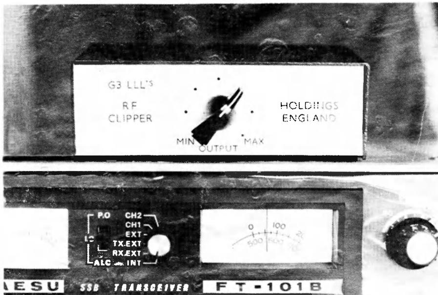
The G3LLL clipper is designed and produced to be compatible with the popular FT101 series of transceivers. It is of course not usable with the new FT101E as this already has an RF speech processor included.
