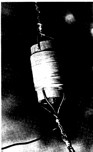
Fig. 2.—Centre loading coil in each dipole.
