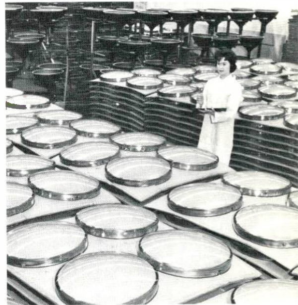
Standing between stacks of phosphor-coated "saucers," Janice White checks inventory of face panels for RCA tubes that will soon produce "living color" TV pictures. Funnels for the tubes, also processed at this RCA Electronic Components and Devices plant in Lancaster, Pa., are shown in the background.
