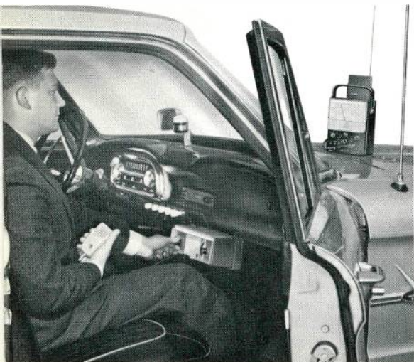
Dick Rainboth, Electronic Instruments Operations, RCA Electronic Components and Devices, demonstrates use of RF-field-strength adapter and V-O-M for checking output of mobile Citizens'-Band equipment.
