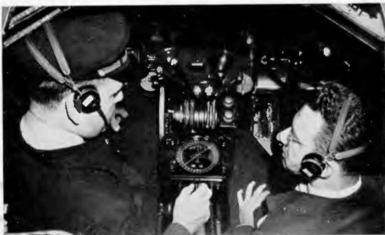
New Sperry-RCA Automatic Direction Finder installed in American Air Lines Douglas Sleeper. Photo shows W. H. Dum, American Air Lines pilot, left, and Lieut. Richard Burke, U. S. Coast Guard, Commander of Coast Guard Air Base at Cape May, New Jersey, discussing the operation of this device after demonstration flight at Floyd Bennett Field on October 12. This Direction Finder, when once tuned to a station, points continuously and automatically at the station so that the pilot need pay no attention to its operation, merely glancing at the pointer on its face
