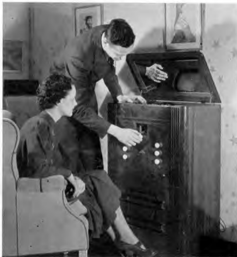
A new photograph of one of the television receiving sets used in connection with NBC's broadcasts of RCA experimental television. Only technicians of the two companies have these sets in their homes. Notice that the television picture is not viewed directly on the screen (properly called Kinescope). It is reflected in the mirror lining of the lid
