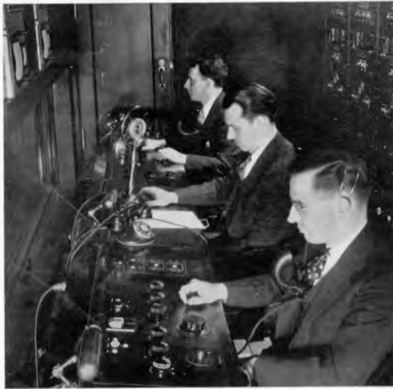
Three engineers man the control room of the NBC experimental television studio in the RCA Building, New York. The engineer in the foreground monitors sound, the one at back monitors the picture. In the center sits the program director, facing a "talk-back" microphone, which connects directly with earphones worn by the men who focus the Iconoscopes in the studio
