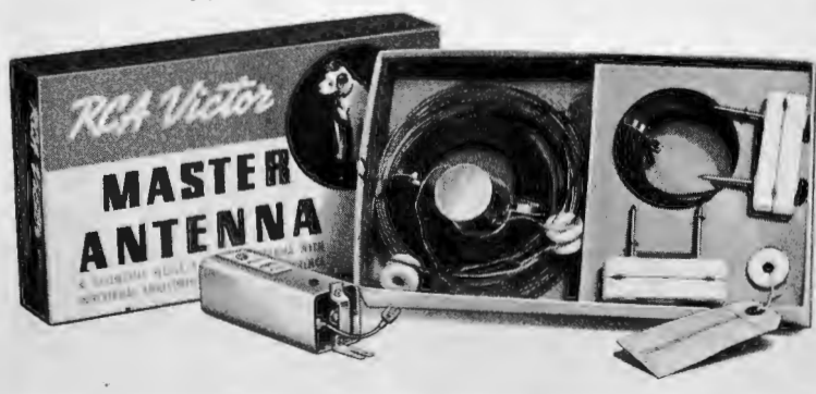
The new RCA Victor Master Antenna differs from the usual noise-reducing antenna in that it employs not only a doublet but also a counterpoise. The counterpoise is adjusted to effectively balance the noise picked up by the entire system
