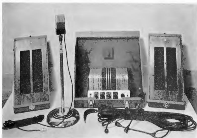
A leader of the new line of RCA Commercial Sound equipment is the PG-112 shown above, a portable outfit of 12-watts undistorted output that lists at only $199.50. Note the chromium finished Junior velocity microphone. The 12-watt amplifier alone has a list price of only $78.60
