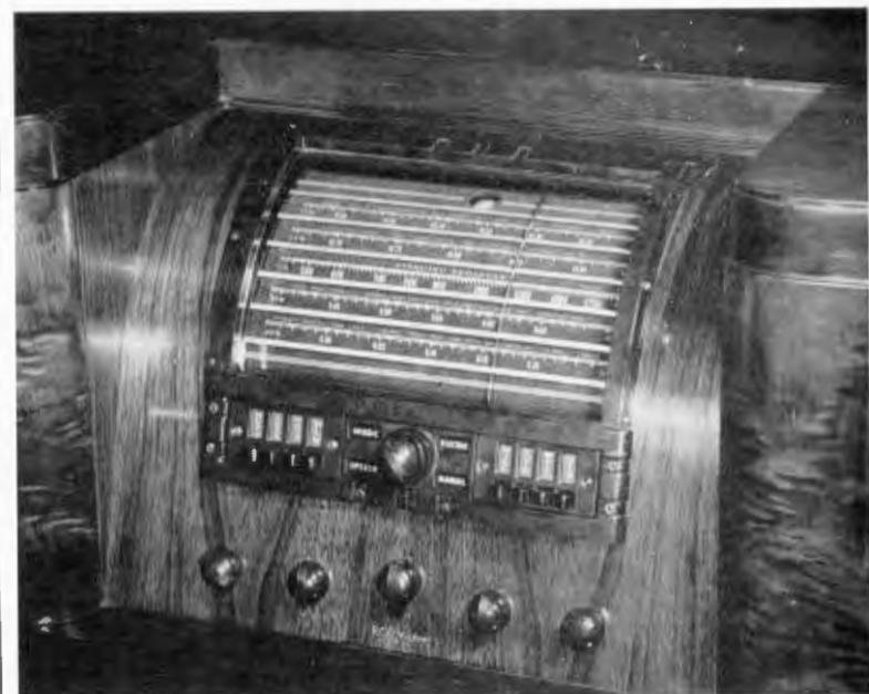
Here is a close-up of two sensational features of the new RCA-Victor line: electric tuning and the new "overseas" dial. Notice the eight tuning buttons with their station designations and the dial above which gives each short wave band a dial space over nine inches long, makes short-wave tuning 50 times easier
