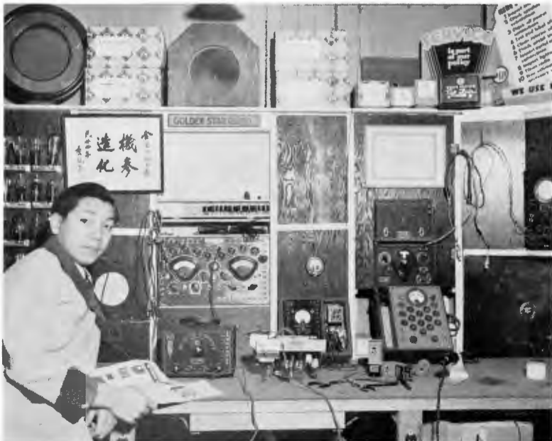
Tommy Tong, owner of the largest Chinese radio shop in the country, is a firm believer in good test equipment. The RCA Beat Frequency Oscillator may be seen in the foreground while the RCA Test Oscillator, Frequency Modulator and Oscillograph are to the right.
