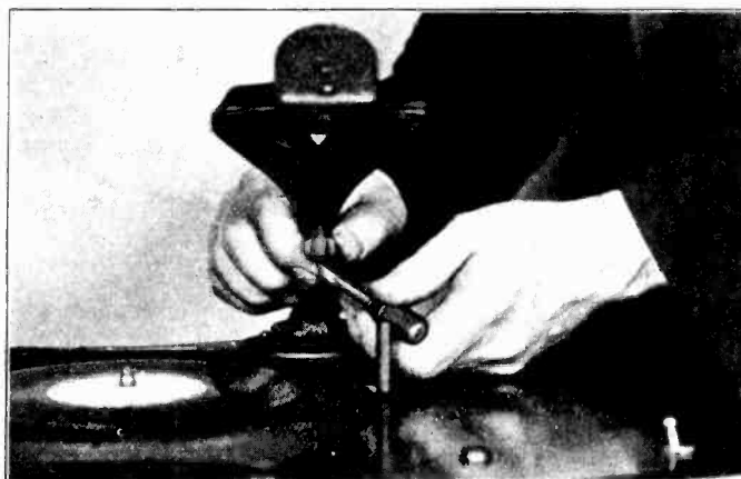
Figure 7—Adjusting Tone Arm Lowering Screw
