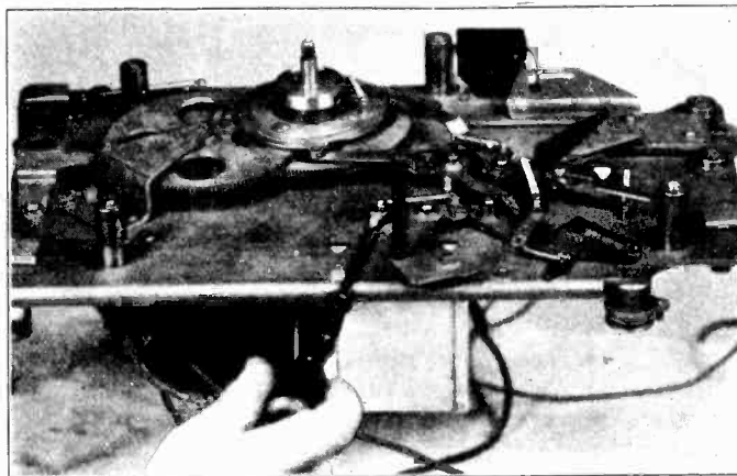
Figure 6—Adjusting Tone Arm Locating Lever
