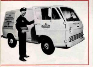
pounds. Ideal for service calls, this light van offers a large, flat floor; double side and rear doors; economical high-torque engine; tough, unitized body frame; flat, broad-view windshield; and underbody areas specially treated to resist rust and corrosion.
