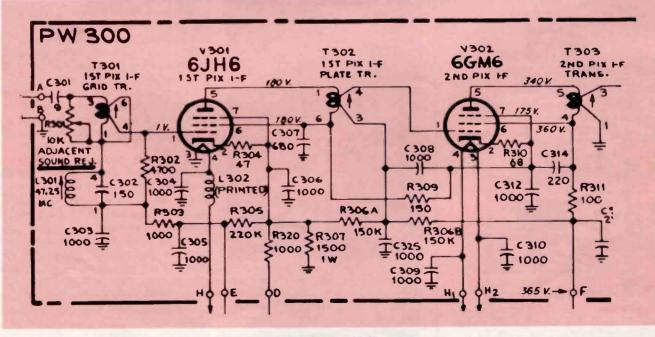
Figure 1: Typical application of bifilar transformers.
