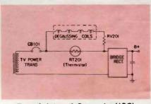
Figure 5: Automatic Degaussing (ADG).
