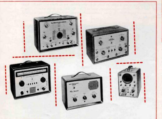
Each Grand Prize in the 1965 Regional Sweepstakes includes these five popular and widely preferred RCA test instruments. Especially suited to color-television servicing, they are (left to right) the WR-99A Crystal-Calibrated Marker Generator, WR-69A Television/FM Sweep Generator, WR-64A Color-Bar/Dot/Crosshatch Generator, WR-70A RF/IF/VF Marker-Adder, and WO-33A Super-Portable 3-Inch Oscilloscope.
