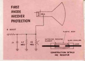
Figure 2: First anode arc-over protection.
