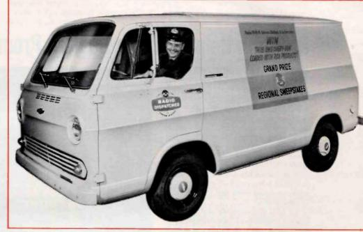
1965 Chevy-Van features 211 cubic feet of load space and a weight capacity up to 2,200 pounds. Double side and rear doors and a large, flat floor make the vehicle an ideal conveyance for delivery and service calls. Operating economy is aided by tough, unitized body-frame construction and an efficient high-torque engine.
