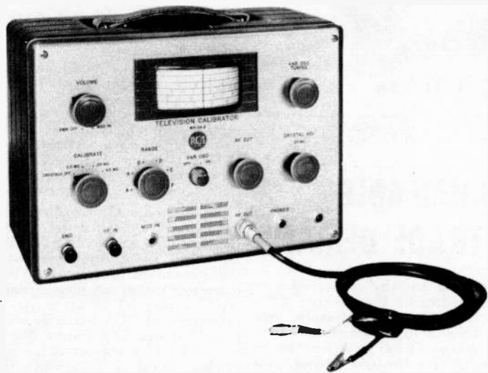
Fig. 1. One of the important functions of the RCA WR-39B Television Calibrator is to serve as a heterodyne frequency meter.
