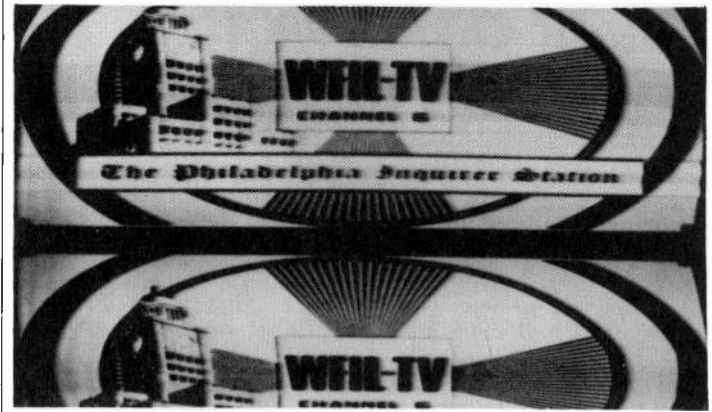
Fig. 2—The presence of two complete pictures indicates that the electron beam in the kinescope is being deflected from top to bottom in 1/30th second, or that the frequency or blocking rate of the vertical oscillator is 30 instead of 60 cycles per second. This condition was produced by increasing the value of the 1.5-megohm resistor in the oscillator grid circuit to 3 megohms, and by adjusting the vertical hold control to obtain a stationary picture. This effect is accompanied by flicker and lack of interlace.
