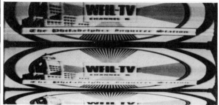
Fig. 3—The presence of three complete pictures indicates that the electron beam in the kinescope is being deflected from top to bottom in 1/20th second, or that the frequency or blocking rate of the vertical oscillator is 20 instead of 60 cycles per second. This condition was produced by increasing the value of the 1.5-megohm resistor in the oscillator grid circuit to approximately 6 megohms and by adjusting the vertical hold control to obtain a stationary picture. This effect is accompanied by flicker and lack of interlace.
