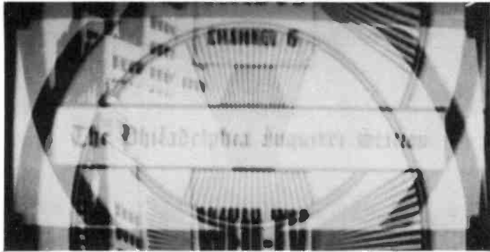
Fig. 4—The presence of two superimposed half-pictures indicates that the electron beam in the kinescope is being deflected from top to bottom in 1/120th second, or that the frequency or blocking rate of the vertical oscillator is 120 instead of 60 cycles per second. This condition was produced by a short circuit across the 1.5-megohm resistor in the oscillator grid circuit and by adjusting the hold control for a stationary picture.
