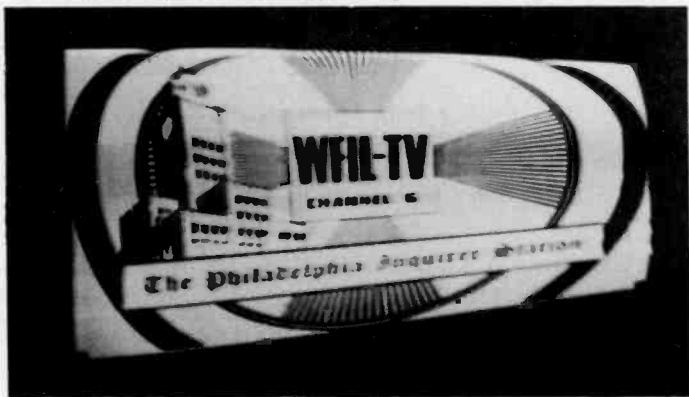
Fig. 5. Same effect as in Fig. 4, but the other half of the vertical deflection coil is shorted, causing keystone in the opposite direction.
