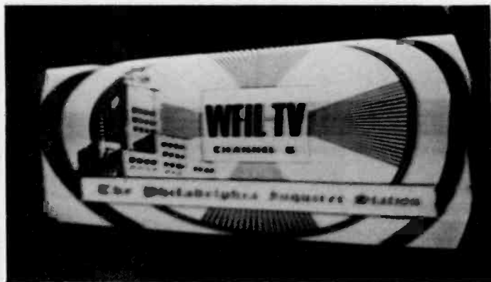
Fig. 4. When the raster or test pattern on a directly viewed kinescope has a trapezoidal or keystone shape, the trouble is usually due to a short circuit or open circuit in the deflection coils. In this photograph, one half of the vertical deflection coil is short circuited.
