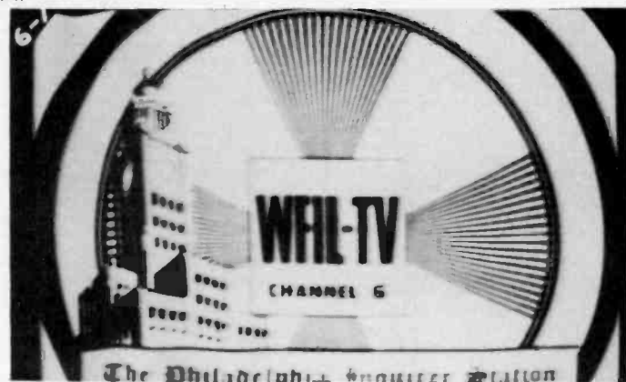
Fig. 8. Damped ripple (ripple of decreasing amplitude) on left half of each horizontal scanning line, produced by open resistors across both sections of the vertical deflecting coil. This damped oscillation occurs in the horizontal deflecting circuit and it is coupled into the vertical deflecting circuit. The resistors across the vertical deflection coils prevent the ripple from becoming evident.
