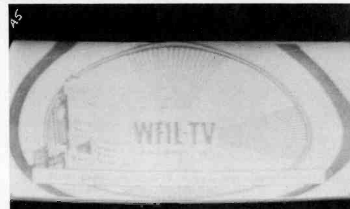
Fig. 11. Insufficient height and poor vertical linearity may be due to incorrect value of the vertical discharge capacitor (0.05 uf), or to open electrolytic capacitors in the cathode and plate circuits of the vertical output tube.
