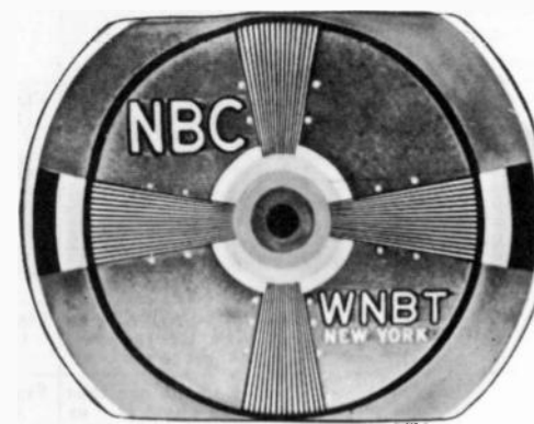
Figure 20—Focus Coil and Ion Trap Magnet Misadjusted
