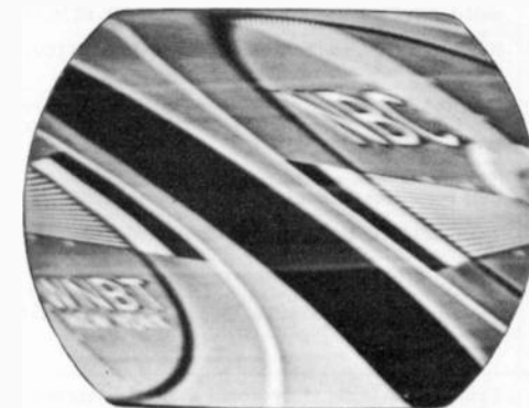
Figure 25—Test Pattern Showing Out of Sync Condition When Horizontal Hold Control Is in a Counter-clockwise Position—Just Before Pulling Into Sync
