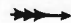
Figure 53—Input of Vertical Deflec- tion Coils (15 Volts PP) (Voltage Across Pins 1 and 2 of J101F)
