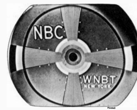
Figure 20—Focus Coil and Ion Trap Magnet Misadjusted
