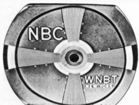
Figure 23—Horizontal Drive Control Misadjusted
