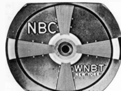
Figure 21—Horizontal Linearity Control Misadjusted (Picture Cramped in Middle)
