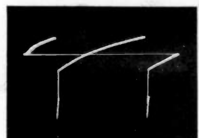
Figure 50—Plate of Vertical Oscillator (Pin 3 of V108) (KCS47 or KCS47A) (Pin 2 of V108B) (KCS47T or KCS47AT) (120 Volts PP)
