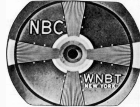
Figure 21—Horizontal Linearity Control Misadjusted (Picture Cramped in Middle)
